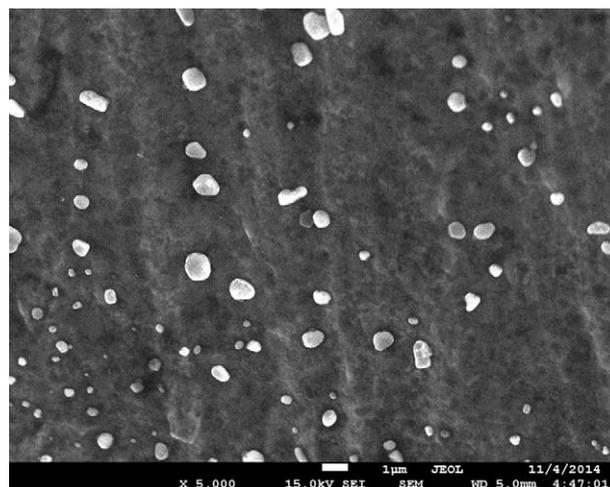
**Figure 3.** Ag-NP present on the Ag-PP-g-PEG-Ti screw (SEM analysis, 1 µm, x5000).
